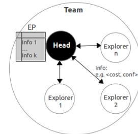
As shown above, a team is composed of one *head node* and several *explorer nodes*, each one being an instance of a Local Search method. Each explorer periodically reports to the head node information on its search process (e.g. its current configuration, the associated cost, the number of iterations reached, the number of local minimum reached, etc.) The *head node* then makes decisions to ensure intensification in the search. To do so, it stores the configurations with the
