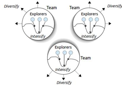
The figure above shows that all available solvers (*Explorers*) are grouped into *Teams*. Each team implements a mechanism to ensure intensification in the search space. Simultaneously, the teams collectively provide diversification for the search. Different teams will work on different regions of the search space. Inter-team communication is needed to ensure diversification while intra-team communication is needed for intensification.
