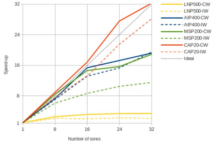
The above figure compares, for each benchmark, the speed-ups obtained with IW (dotted line) and CW (continuous line). In most cases, CW is getting closer to the “ideal” speedup. For instance, in CAP the cooperative strategy actually reaches super linear speed-ups over the entire range of cores (speed-up of 32.2 with 32 cores). The best gain reaches 69% in the MSP.
