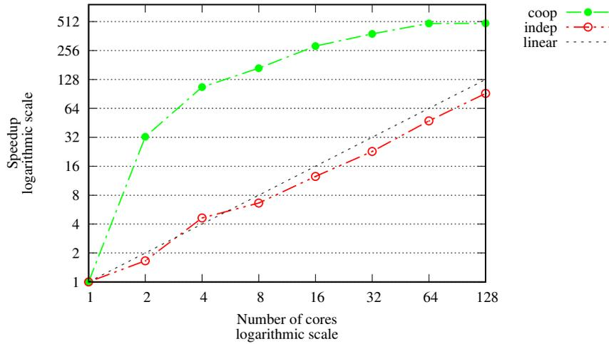
Fig. 7 Speedups obtained with AS-SMTI on hard instances of SMTI problems (size = 1 000)
