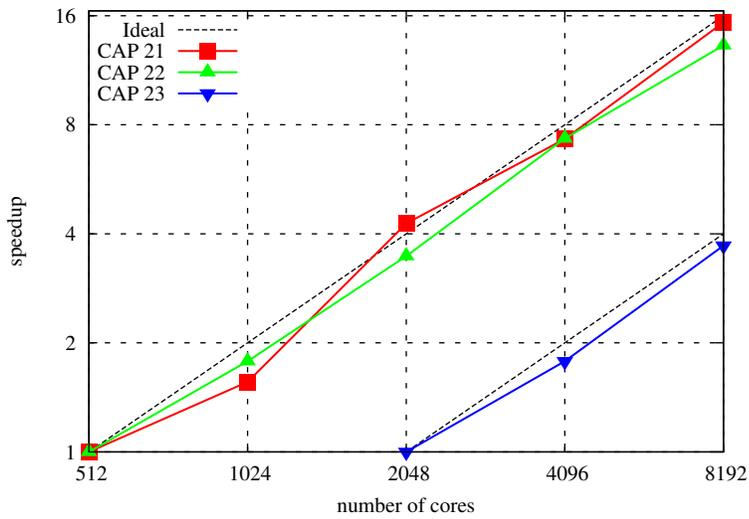
**Fig. 5** Speedups for the Costas Array Problem on the JUGENE supercomputer, from [29]
