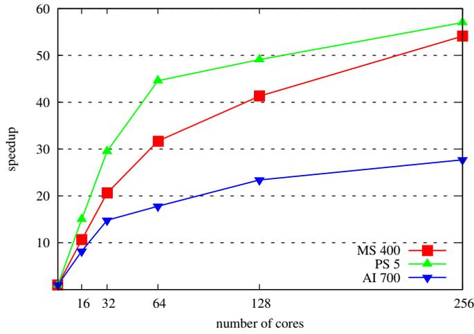
**Fig. 4** Speedups for benchmark CSP programs on the HA8000 parallel machine, from [28]
